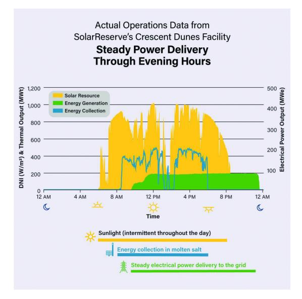
**4. Lighting up the night.** Using sensible heat storage, the Crescent Dunes project is able to produce energy long after the sun has set, helping power the lights of Las Vegas. *Courtesy: SolarReserve*
